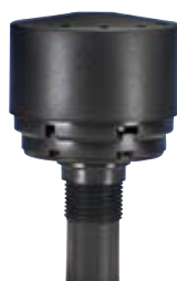
AD-12 Automatic Drain Valve (Internal) Temp: 175°F (79°C) Pressure: 10-250 PSIG (17 bar) 1/8" NPT Drain Connection
