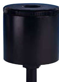
MS-50 Metal Sump Drain (External) Temp: 175°F (79°C) Pressure: 10-250 PSIG (17 bar) 1/2" NPT Inlet Connection 1/8" NPT Drain Connection
