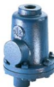
ADT-50 Float Actuated Drain Trap Temp: 450°F (232°C) Pressure: 150 PSIG (10 bar) 1/2" NPT Inlet Connection 1/4" NPT Drain Connection
